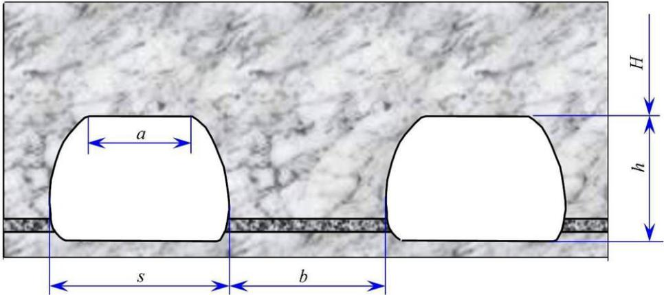
**Fig. 8.** To calculation of long safety pillar width.
