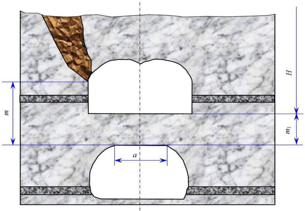
**Fig. 6.** Development of disturbed gypsum seam at two levels.
