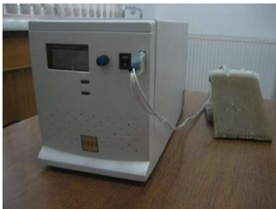
სურ.2. Apparatus for therapy of proctologic (rectum) and cervic uterus cancer diseases by local controlled carcerthermia method – “LEZI”. Certificate 6374. 2015. Georgian Patent. “saqpatenti”.
