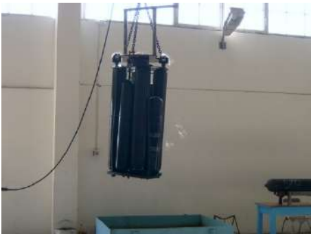
Fig. 4. Cooling the cylinders in the tank for hardening.
