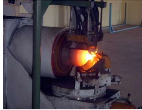
Fig. 2. Deformation at the end of the pipe.
