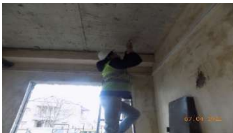
Fig. 7. Determination of r/c slab concrete strength
