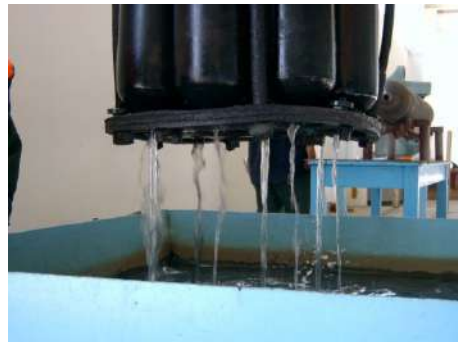
Fig. 4. Cooling the cylinders in the tank for hardening.
