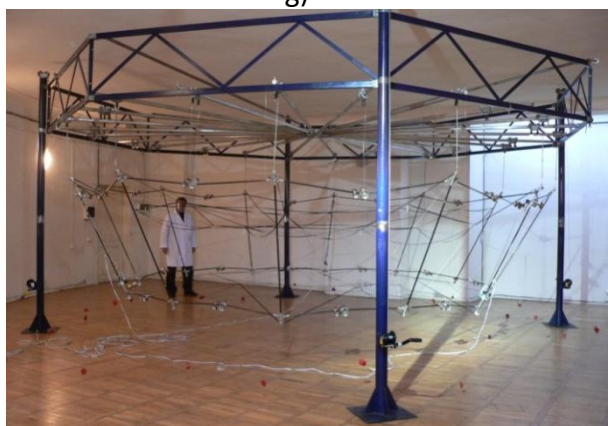
fig. III.41 _ wakveTili piramidis formis mqone, „Casatex“ Reroebiani, zambarebiT gasaxsnel rgoliani da moqnili, gaWimul centriani gasaSleli kosmosuri refleqtoris gaSlis fotociklogramma
