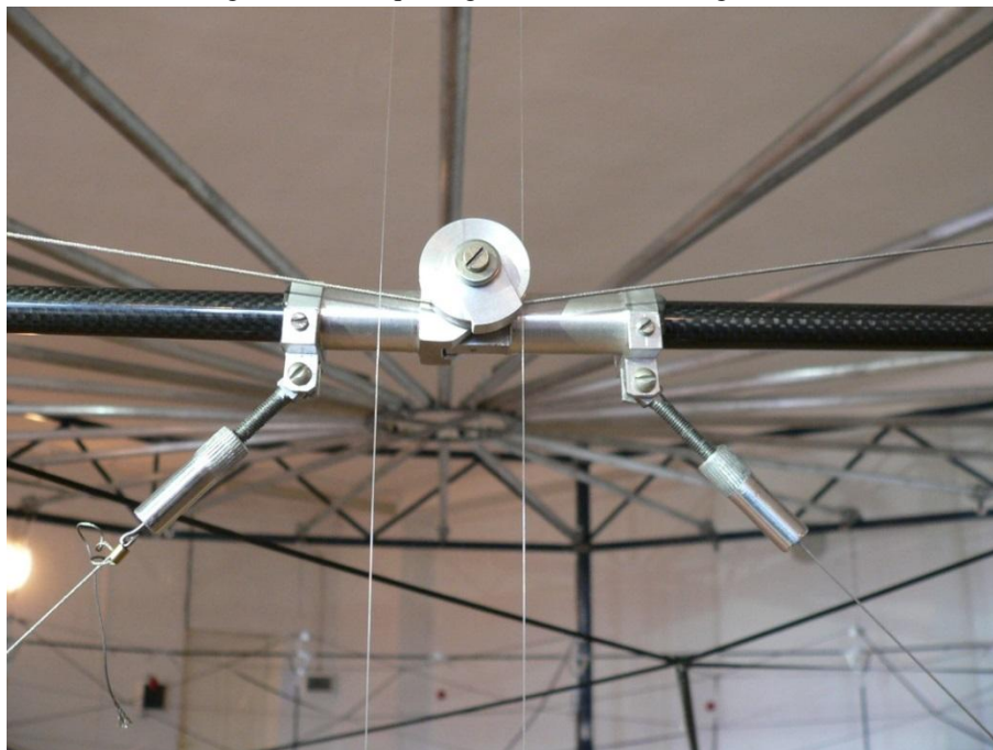
fig. IV.2 _ zeda sartyelis mosazRvre berketebi erTiandebian cilindrul saxsarSi, romlis Reroebzec wamocmulia gorgolaWi, romelzec Semotarebulia rgolis gamSleli Zalovani bagiri. saxsris siaxloves aseve tendebiT Camagrebulia rgolis geometriuli ucvlelobis mimniWebeli, rombis formiT ganTavsebuli vantebi, romlis meore boloebi dgaris Sua wertilzea mimagrebuli.
