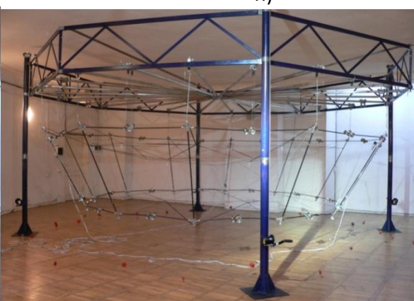
fig. III.41 _ wakveTili piramidis formis mqone, „Casatex“ Reroebiani, zambarebiT gasaxsnel rgoliani da moqnili, gaWimul centriani gasaSleli kosmosuri refleqtoris gaSlis fotociklogramma
