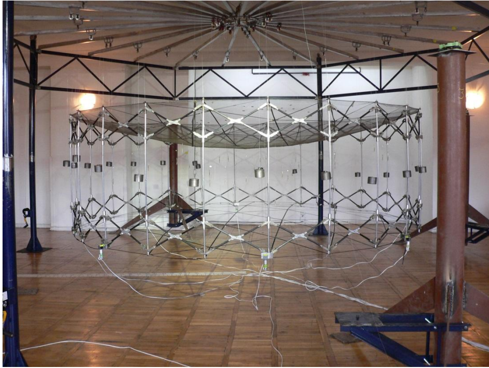
fig. III. 11 _ or rigad ganTavsebuli pantografuli struqturis gamSlelrgoliani da moqnili, gaWimulcentriani gasaSleli refleqtoris 4 metri diametris funqionaluri modelis transformaciebi dakecili mdgomareobidan misi gaSlis CaTvliT.
