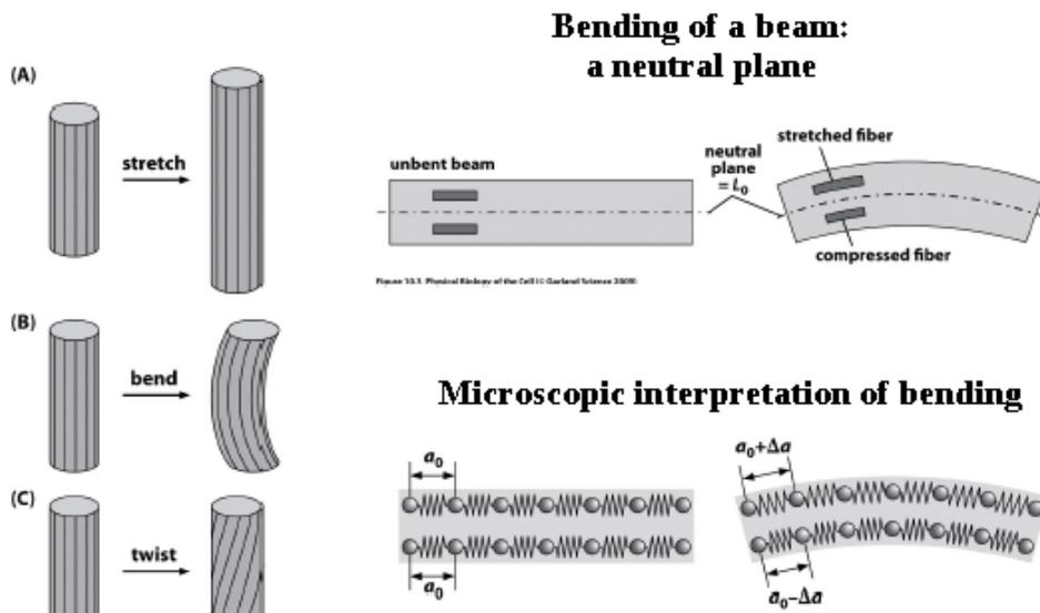
Figure 10.32. Three types of deformations.
