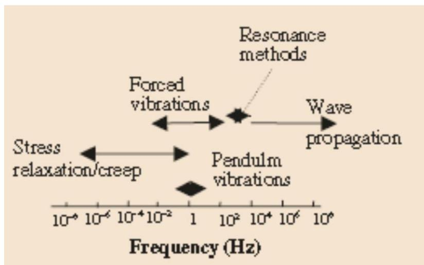
Figure 15.40. Methods for the measurement of the linear viscoelasticity of solid materials over different frequency ranges.[Ref.: Becker, Mater. Plast. Elast., 1969, 35, 1387].
