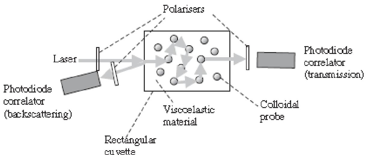
Figure 15.37 Schematic diagram of a diffusing wave spectroscopy experiment. (Coherent laser light is multiply-scattered from a dense suspension of colloidal particles. Analysis of the resultant correlation functions can provide the high frequency viscoelasticity of a biological specimen).
