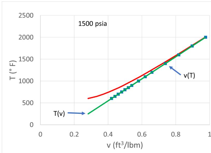
Figure 6.1. Steam table data with ideal gas approximation calculations for 4000 psia. The red line represents the actual  $v - T$  data from the superheated tables for water, while the green line represents temperatures calculated from tabulated pressure and specific volume data using the ideal gas approximation, and the blue symbols represent specific volumes calculated from tabulated pressure and temperature data.
