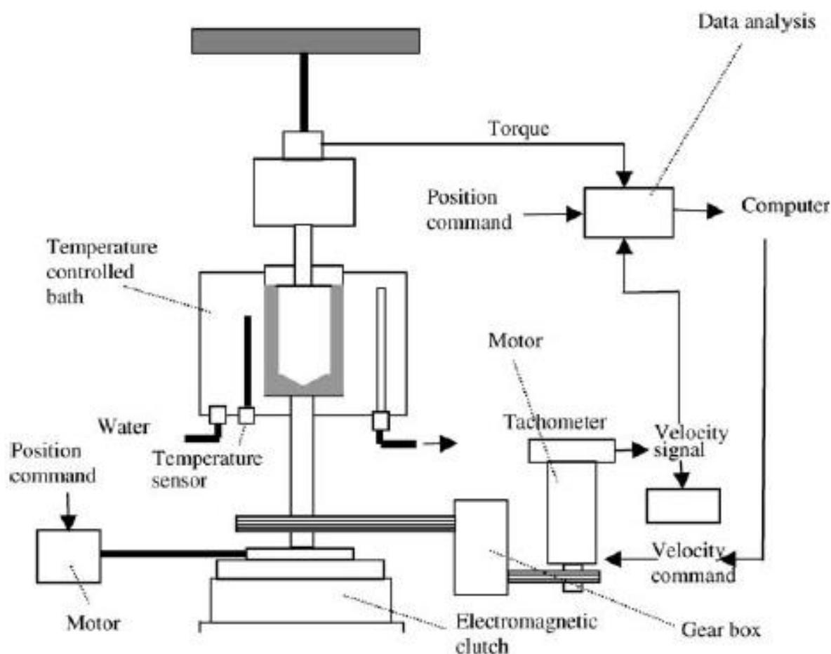
Figure 15.32 Schematic diagram of a modern shear rheometer. [Ref.: L. Bohlin, in Progress in Trends in Rheology, II, Eds H. Gieseku and M.F. Hibberd, Steinkopf, 1988, 151].
