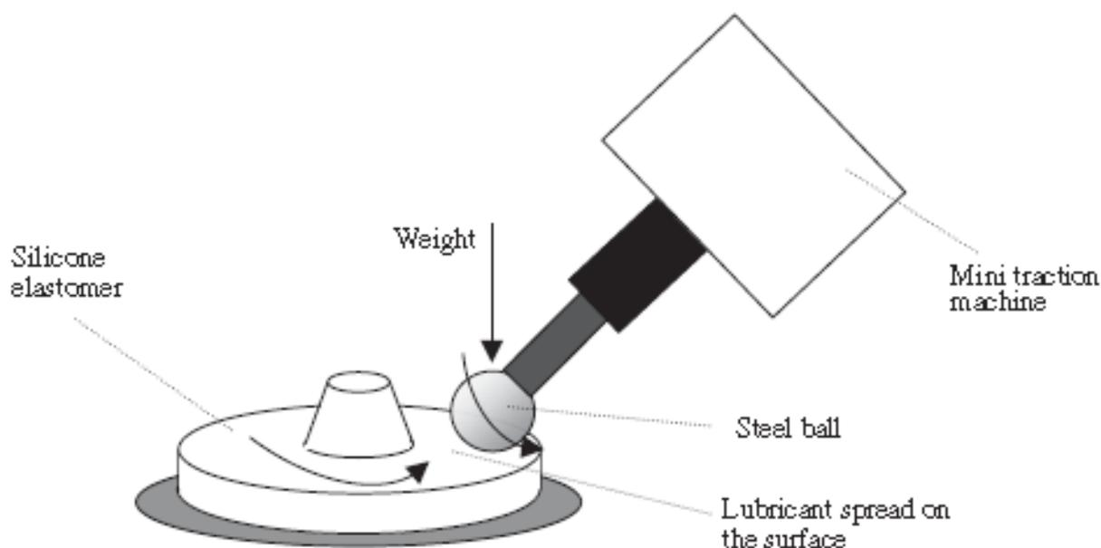
Figure 15.39. Modern ball on plate tribometer used to measure the friction coefficient of thin viscoelastic films as a function of shear rate (Stribeck curves). [Ref.: J. de Vicente, J.R. Stokes and H.A. Spikes, *Tribology International*, 2005, 38, 515–526].
