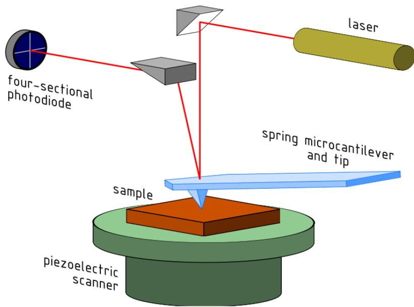
Figure 15.17 Detailed schematic diagram of an AFM apparatus. The feedback scheme can be used to hold the cantilever at a constant force on the sample. [Ref.: J.Yang, L.K.Tamm, A.P. Somlyo and Z. Shao, *Journal of Microscopy*, 1993,171, 183–198].
