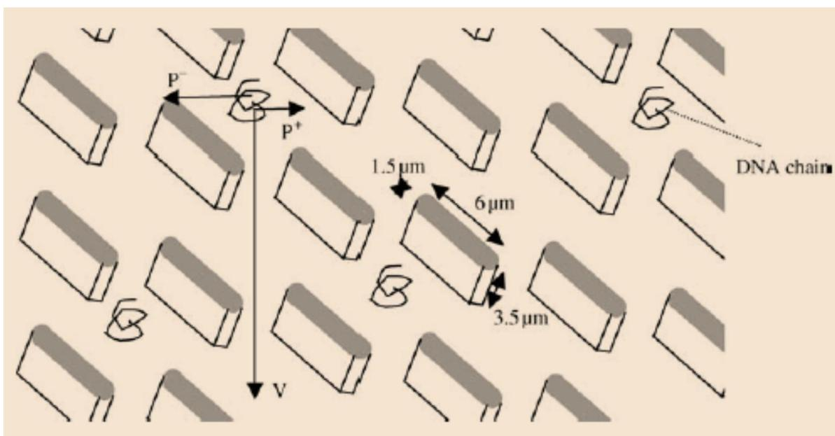
Figure 15.26. Etched microarrays used for electrophoresis experiments. (An electric field moves the DNA molecules vertically downwards with a velocity  $v$ . Due to the anisotropic nature of the obstacle orientation there is a larger probability for the molecules to change channels to the right ( $P^+$ ) than to the left ( $P^-$ ), and this probability is a function of the size of the chains [Ref.: C.F.Chou, R.H.Austin, O.Bakajin et al., *Electrophoresis*, 2000, 21, 81–90]
