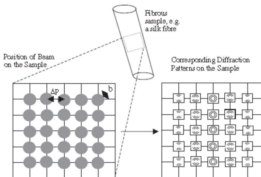
Figure 15.2 Scanning X-ray microdiffraction across a semi-crystalline anisotropic Material ( $b$  is the diameter of the X-ray beam). Two dimensional diffraction images are recorded at micron spaced steps ( $\Delta p$ ) across the sample and provide detailed information on the molecular structure of the fibres.
