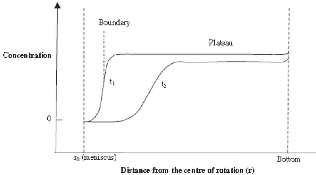
Figure 15.29. Schematic diagram showing the progress of a moving boundary sedimentation experiment at two different time steps ( $t_1$  and  $t_2$ ). The boundary moves towards the centre of rotation (the cell bottom) as a function of time.
