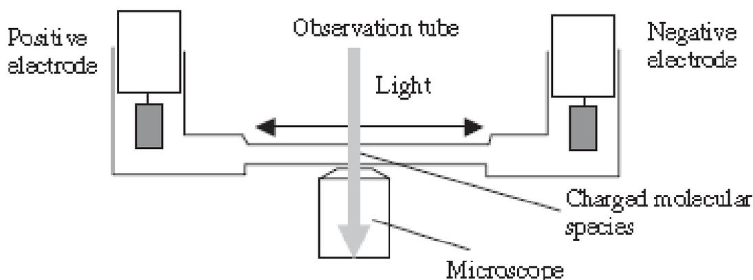
Figure 15.20. A moving boundary apparatus for the examination of free solution electrophoresis. The motion of the colloids that experience electrophoresis is measured with an optical microscope.
