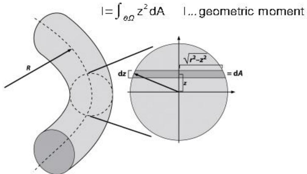
Figure 10.34. Precise calculation of the total strain energy of the beam.
