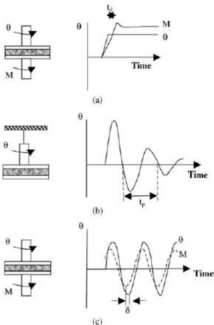
Figure 15.33. Methods for the measurement of the shear modulus: (a) wave speed, (b) resonance and (c) forced oscillations [Adapted with permission from C.W. Macosoko, *Rheology, Principles, Measurements and Applications*, Copyright (1994) Wiley-VCH].
