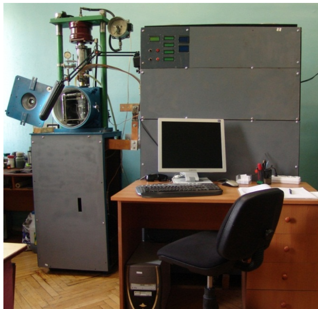
Fig.5. SPS device designed and built by our team in the RCSR at the Georgian Technical University
