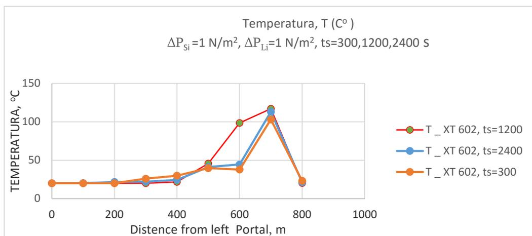
Fig.12. Dynamics of changes the spatial scale of Temperature along the tunnel. The simulation time is  $t_s = 300 \text{ s}$ ,  $1200 \text{ s}$ ,  $2400 \text{ sec}$ .
