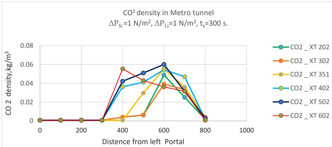
Fig. 6. Dependence of distribution of carbon dioxide concentration in the tunnel of the subway on the forced stop location of train. (HRR = 30 MW, height  $Z = 1.5$  along the tunnel, simulation time 300 seconds)
