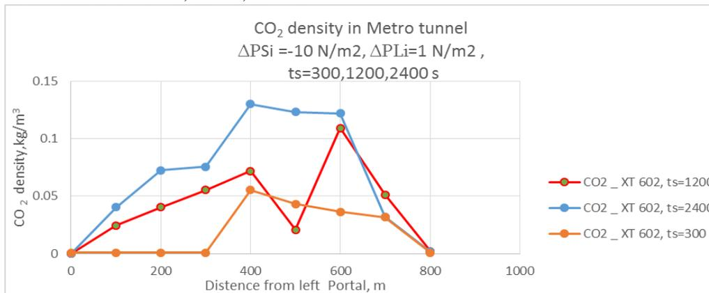
Fig. 10. Dynamics of changes the spatial scale of concentration increase of carbon dioxide along the tunnel. The simulation time is  $t_s = 300\text{ s}$ ,  $1200\text{ s}$ ,  $2400\text{ sec}$ .
