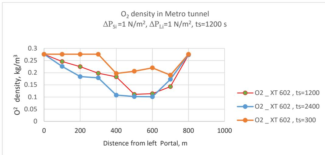
Fig. 11. Dynamics of changes the spatial scale of concentration decrease of Oxygen along the tunnel. The simulation time is  $t_s = 300\text{ s}$ ,  $1200\text{ s}$ ,  $2400\text{ sec}$ .
