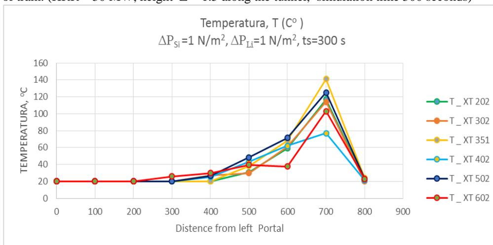
Fig. 8. Dependence of distribution of Temperature in the tunnel of the subway on the forced stop location of train. (HRR = 30 MW, height  $Z = 1.5$  along the tunnel, simulation time 300 seconds)
