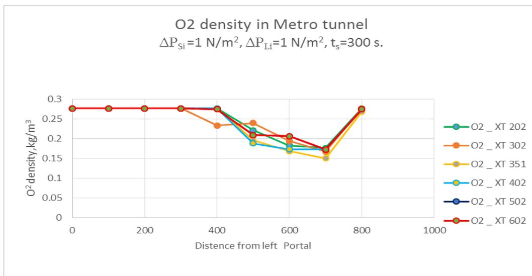
Fig. 7. Dependence of distribution of oxygen concentration in the tunnel of the subway on the forced stop location of train. (HRR = 30 MW, height  $Z = 1.5$  along the tunnel, simulation time 300 seconds)
