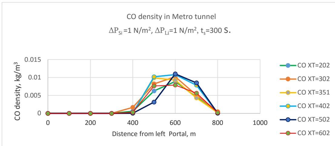
Fig. 5. Depends of distribution of carbon monoxide concentration in the tunnel of the subway on the forced stop location of train. (HRR 30 MW, height  $Z = 1.5$  along the tunnel, simulation time 300 seconds)
