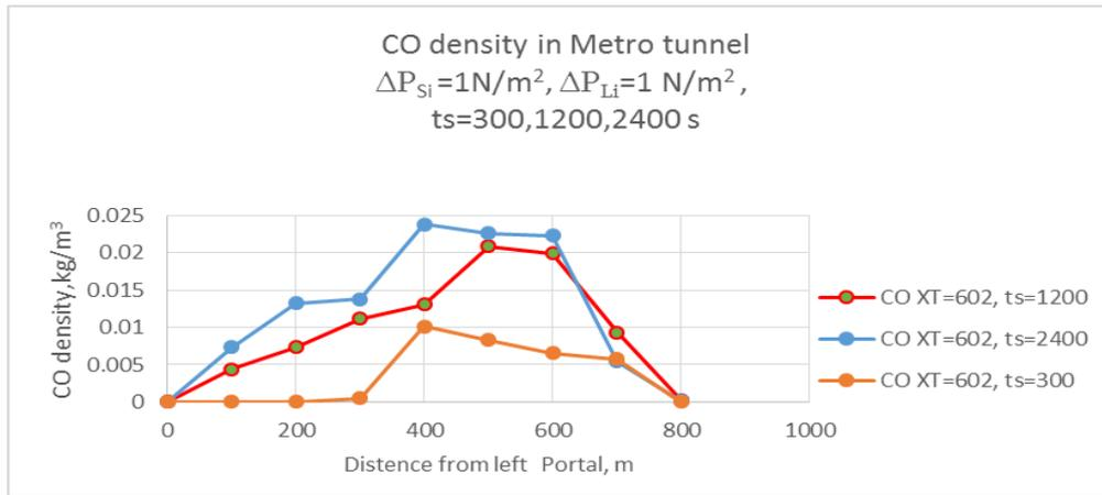
Fig.9. Dynamics of changes the spatial scale of concentration increase of carbon monoxide along the tunnel. The simulation time is  $t_s = 300\text{ s}$ ,  $1200\text{ s}$ ,  $2400\text{ sec}$ .
