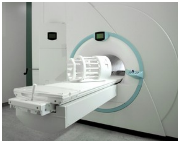
9.4-tesla magnetic resonance tomograph (MRT) combined with a positron emission tomograph (PET).
