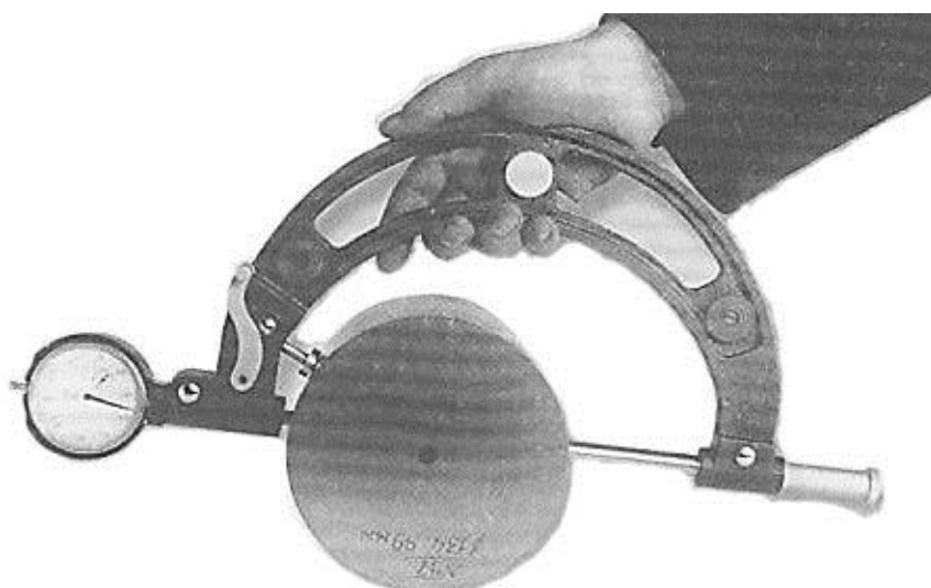
Fig. 1. The measuring of journal neck diameter by lever external gauge
